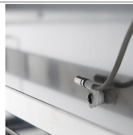
Internal cell probe for constant temperature monitoring
