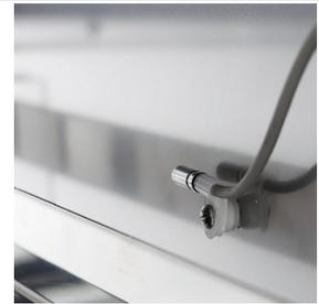
Internal cell probe for constant temperature monitoring
