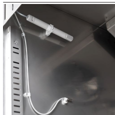
Humidity control with electronic probe
