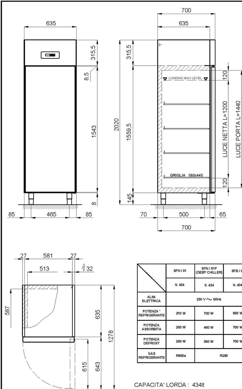
Technical drawings showing front, side, and top views of the refrigerator with dimensions in millimeters. Front view shows a width of 635mm and a height of 1543mm. Side view shows a depth of 700mm and a height of 2020mm. Top view shows a width of 635mm and a depth of 587mm.
