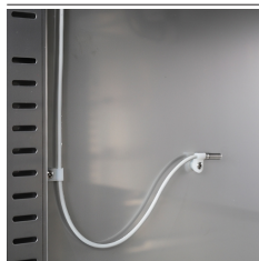
Internal cell probe for constant temperature monitoring
