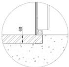
Scheme for floor recessed installation
