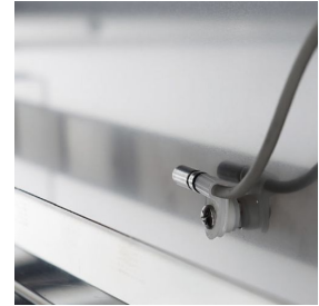
Internal cell probe for constant temperature monitoring
