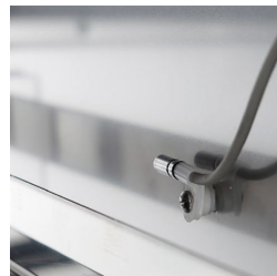
Internal cell probe for constant temperature monitoring
