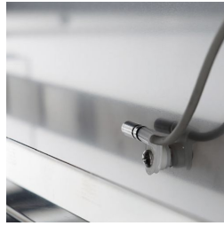
Internal cell probe for constant temperature monitoring
