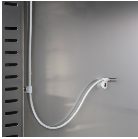
Internal cell probe for constant temperature monitoring
