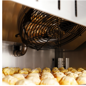
Evaporators with cataphoresis treatment and electronic fans
