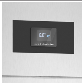
Control electronic board for the constant management of temperature and relative humidity
