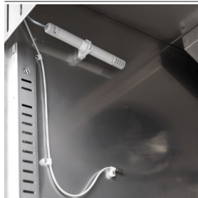
Humidity control with electronic probe
