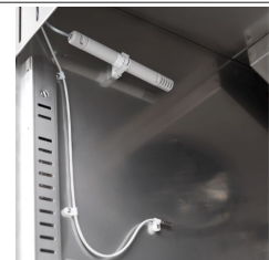
Humidity control with electronic probe
