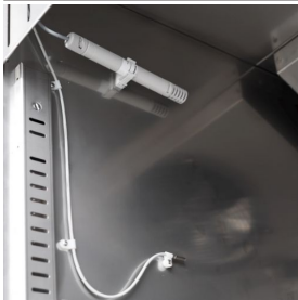
Humidity control with electronic probe
