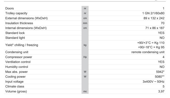
\*Evap. -10°C, Cond. +45°C / \*\*Evap. -23,3 Cond. +54,4°C \*\*\*Ambient temp. +30°C loading sample according to EN 17032:2018
