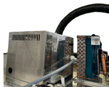
High-efficiency steam boiler (steam production from 2-2.6 kg/h).
