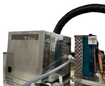
High-efficiency steam boiler (steam production from 2-2.6 kg/h).
