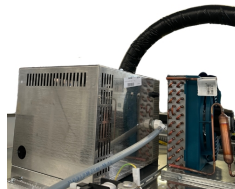
High-efficiency steam boiler (steam production from 2-2.6 kg/h).
