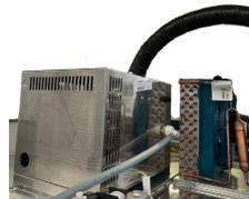
High-efficiency steam boiler (steam production from 2-2.6 kg/h).
