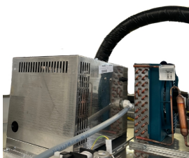
High-efficiency steam boiler (steam production from 2-2.6 kg/h).
