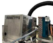
High-efficiency steam boiler (steam production from 2-2.6 kg/h).
