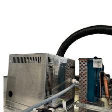
High-efficiency steam boiler (steam production from 2-2.6 kg/h).
