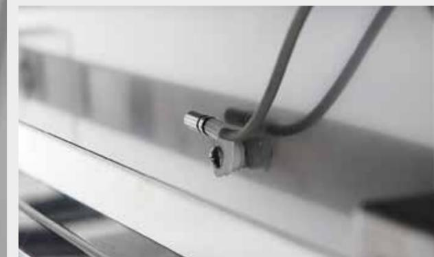
Internal probe for constant temperature control.
